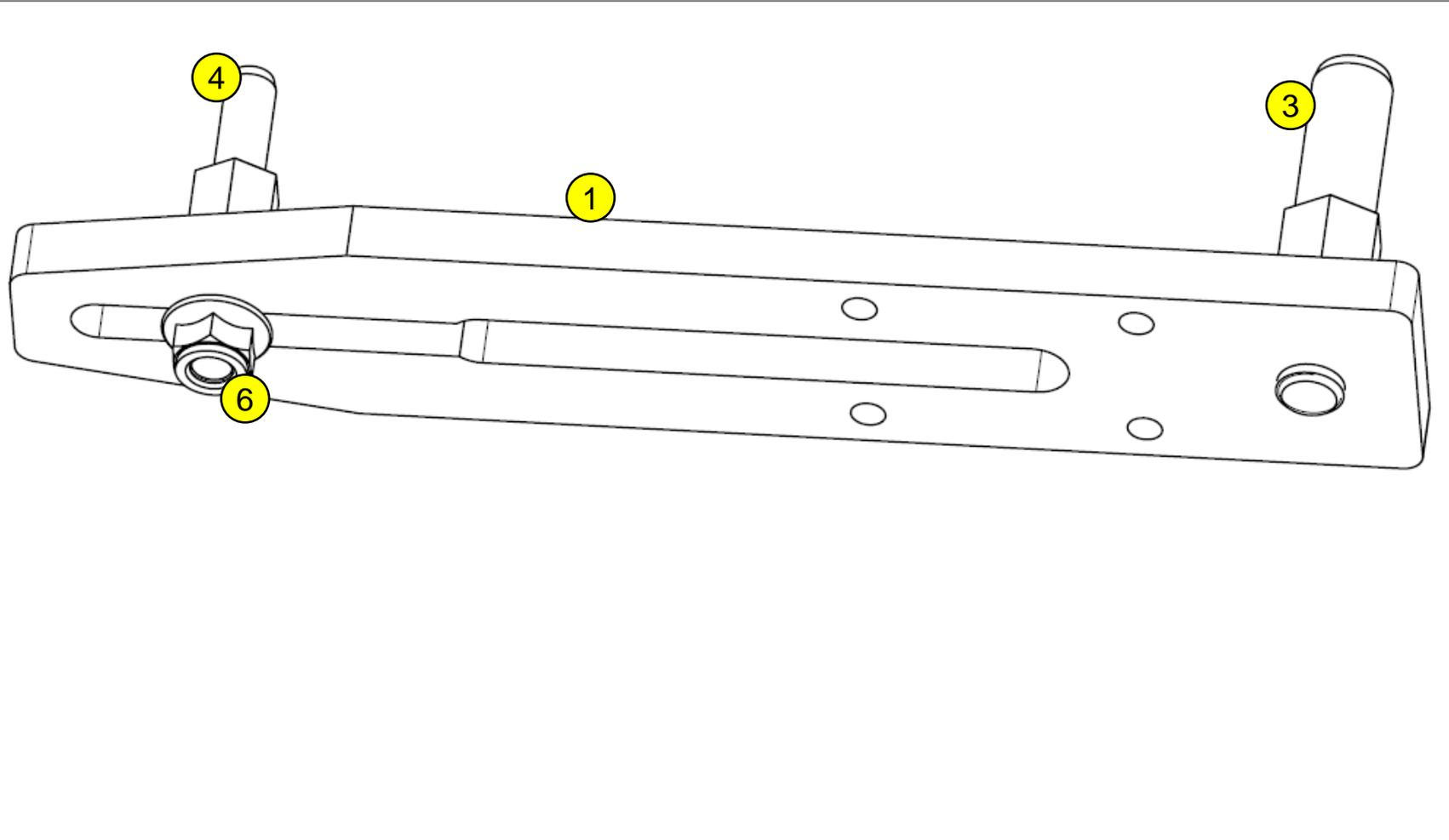
1. Screw the upper pin (3) to the adapter plate (1).
