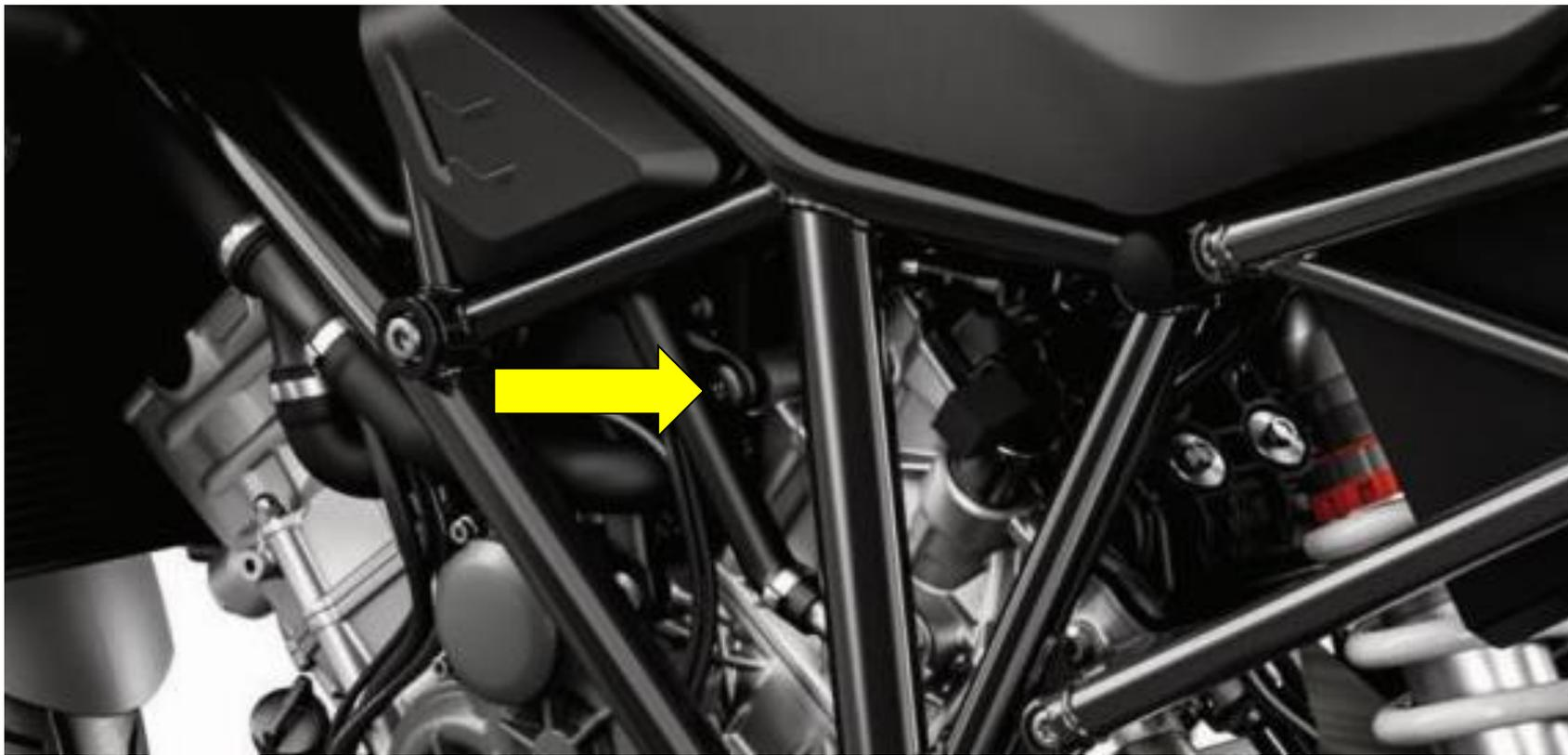
Remove the screw in the direction of the arrow.
