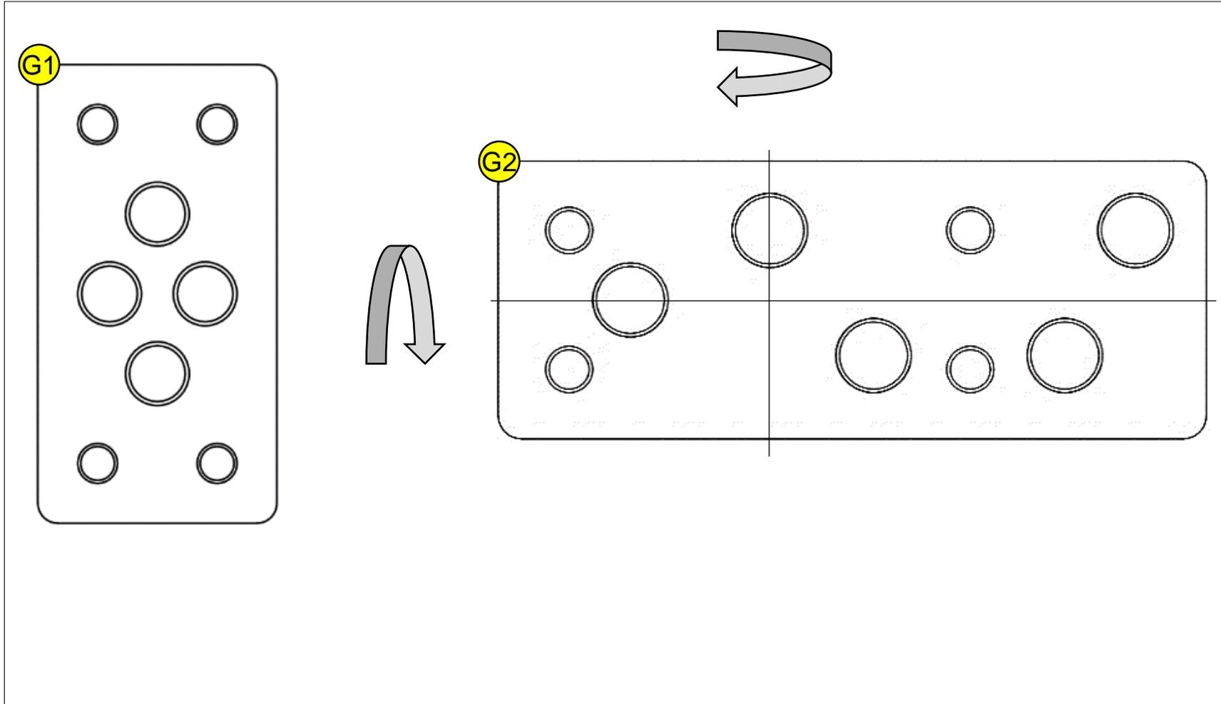
For optimum alignment of the adapter plate on the base plate **G1**, an extended base plate **G2** is available; the extended base plate can be rotated by 180°.
