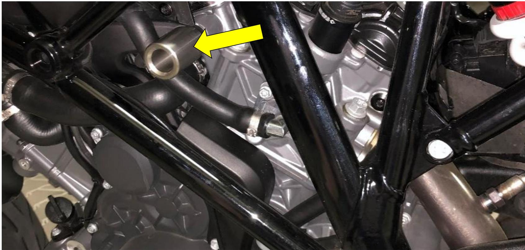
Use the cylinder head screw ⑤ to screw the frame sleeve ② to the frame.
